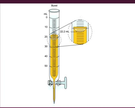
Read volume at the bottom of the liquid curve
