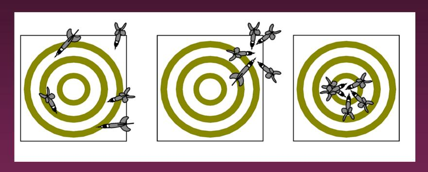
Neither precize nor accurate Precize but not accurate Both precize and accurate
